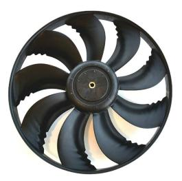
The 30RB-RBP/30RQ-RQP unit uses Carrier's sixth generation Flying Bird<sup>™</sup> fan technology, engineered for maximum efficiency, super low noise, and a wide operating range. The fans use Carrier patented rotating shroud technology and back-swept blades with a wave-serration trailing edge inspired by nature.
