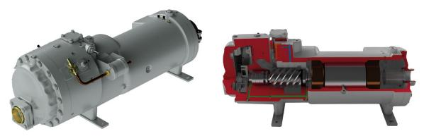
The new generation of 06Z variable-speed twin screw compressors benefits for Carrier's long experience in the development of twin-rotor screw compressors. The 06Z compressor design is based on the successful 06T screw compressor, core of the well-known Aquaforce series with a number of modifications to reduce noise level and improve the energy efficiency especially during part load operation.
