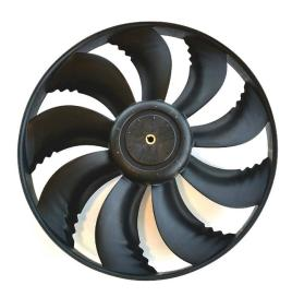
The 30KAVZE/30KAVPZE utilizes Carrier's the 6th generation Flying BirdTM fan technology, engineered for maximum efficiency, super low noise, and wide operating range. The fan includes Carrier patented rotating shroud technology and back-swept blades with a unique wave-serration trailing edge inspired from nature.
