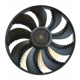
The 30RB/30RQ unit uses Carrier's sixth generation Flying Bird<sup>TM</sup> fan technology, engineered for maximum efficiency, super low noise, and a wide operating range. The fans use Carrier patented rotating shroud technology and back-swept blades with a wave-serration trailing edge inspired by nature.
