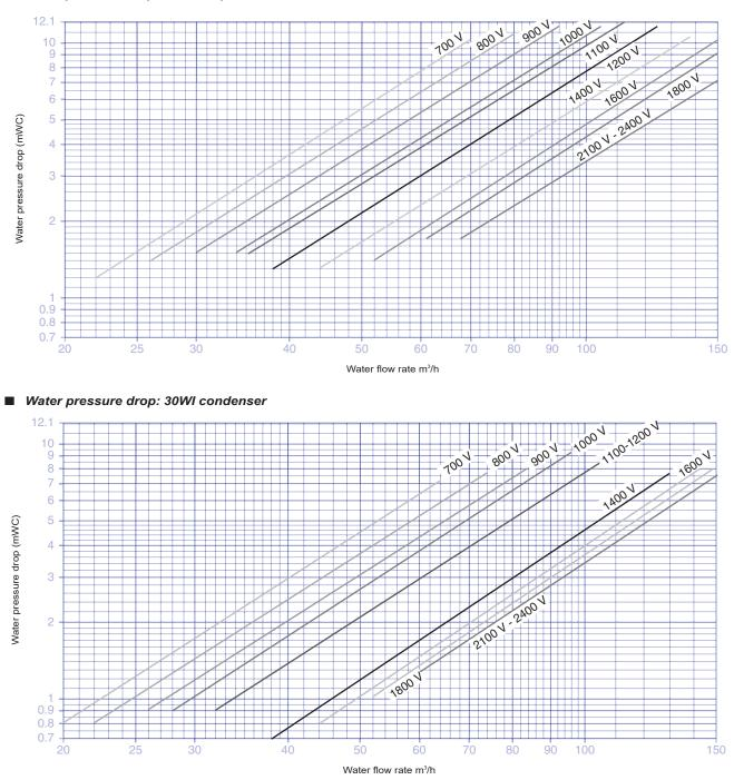
■ Water pressure drop: 30WI evaporator
