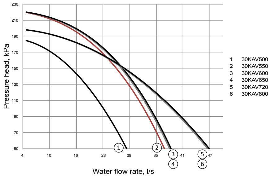
**High-pressure variable-speed dual pump
