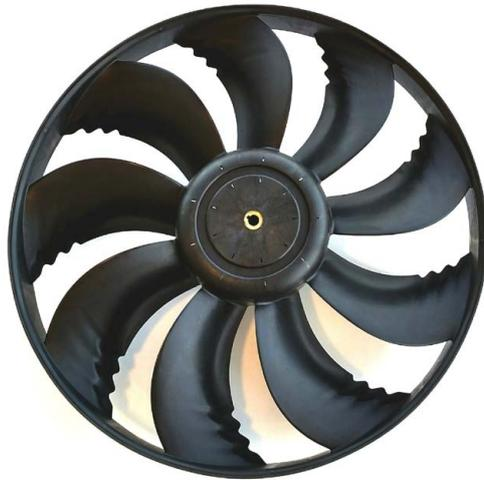
The 30KAV utilizes Carrier's the 6th generation Flying Bird™ fan technology, engineered for maximum efficiency, super low noise, and wide operating range. The fan includes Carrier patented rotating shroud technology and back-swept blades with a unique wave-serration trailing edge inspired from nature.
